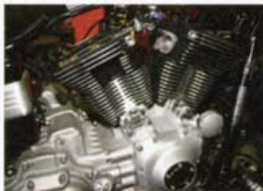
The cylinders and heads bolted on just as with the stock parts. They required no custom fitting or machining. Revolution Performance supplied custom head gaskets made by Cometic.
