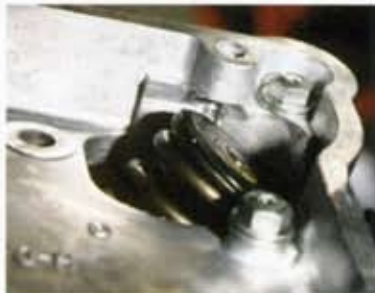
The Bill Chambers Racing cylinder heads use high-performance valve springs and full size retainers.
