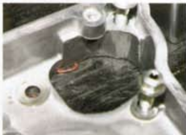
Larry had to grind the area just inside the rocker box where each valve spring retainer sits. This was the only custom fitting required in the whole installation. The throttle body and exhaust systems were straight bolt-on propositions.
