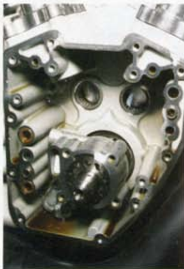
The 2006 Dyna models and all 2007 Twin Cam motors have larger inner cam bearings and a higher capacity oil pump. Camshafts made for the earlier motors will not work in the new motors.
