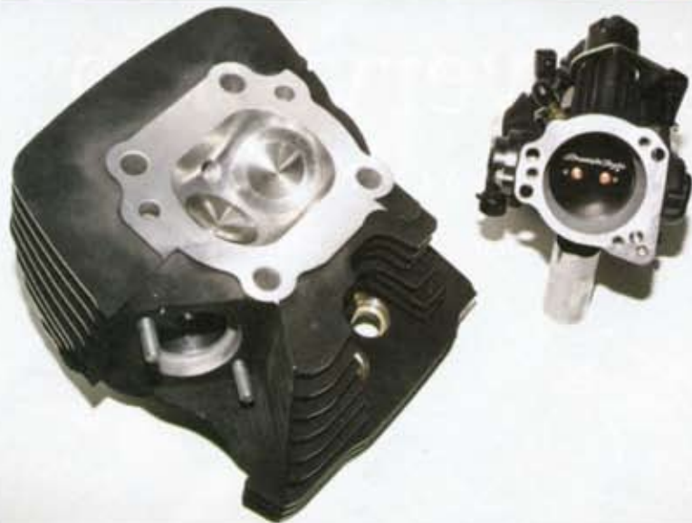
We matched Harley's 50mm Screamin' Eagle throttle body with a set of Twin Cam cylinder heads that had been reworked by Bill Chambers Racing. The throttle body comes with high-flow injectors and all the electronic sensors installed. The heads have 1.900-inch intake and 1.610 exhaust valves.
