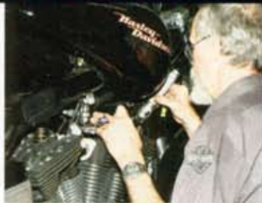
When Larry fitted the rocker boxes, he found that the valve spring retainers contacted their inner walls.
