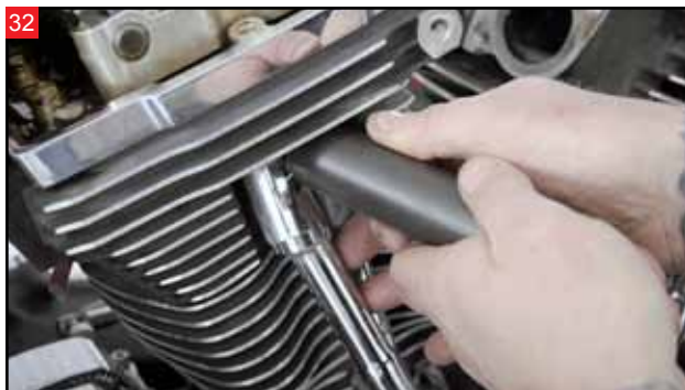
To access the pushrods, remove the top clips from the pushrod tubes. Use a center jack under the frame to raise the rear wheel off the lift.
