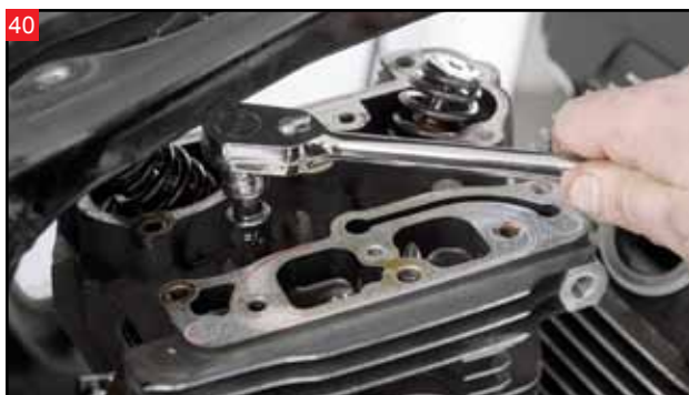
40 With a 1/2" 12 point socket, break the four head bolts loose.
