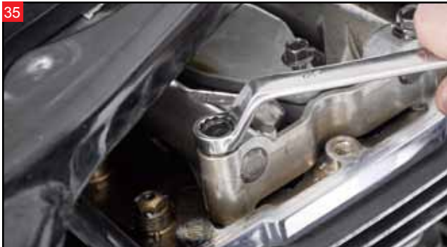
Loosen the four bolts holding the rocker arm pedestal with a 1/2" wrench.
