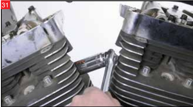
With a 3/4" deep well socket, the engine temperature sensor can be removed from the front cylinder head.
