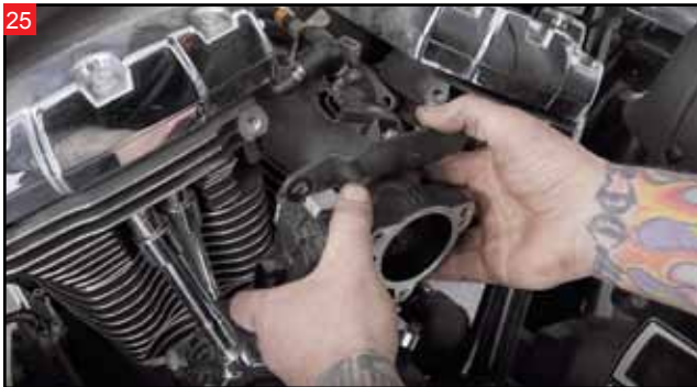
Remove the throttle body from in between the cylinder heads from the right side of the motorcycle.
