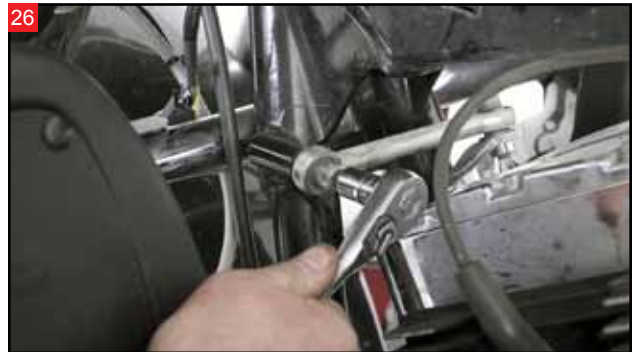
With a T45 Torx driver, remove the bolt holding the front motor stabilizer link to the frame.
