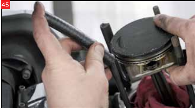
45 Slip the 3/8" rubber hose over the outside cylinder studs for the pistons to rest on. This will help prevent damage to the piston or cylinder stud.
