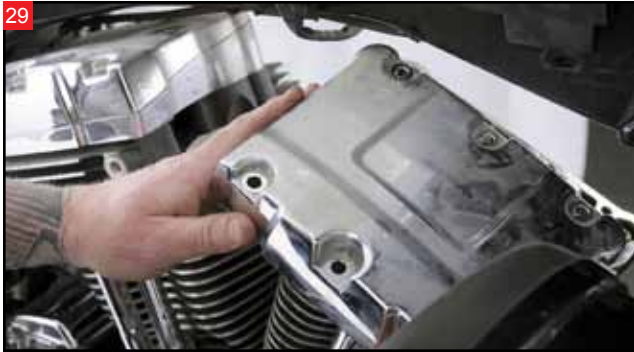
Remove the rocker box top and gasket from the lower rocker box housing. Repeat the process for the other rocker box.
