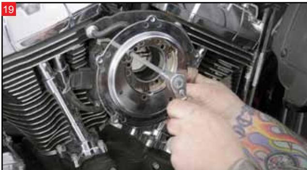
With a 3/16" Allen, remove the three bolts holding the backing plate to the throttle body.
