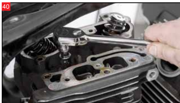
With a 1/2" 12 point socket, break the four head bolts loose.
