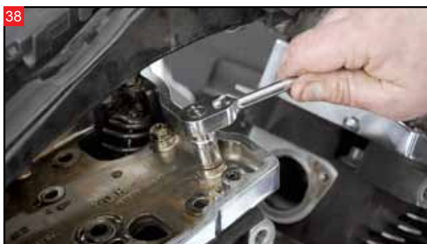
38 Loosen the six bolts holding the lower rocker housing to the head.
