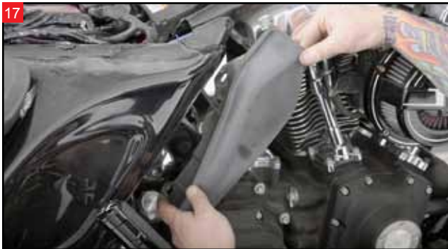
Use a 7/16" socket to remove the hardware holding the heat guards from the frame.
