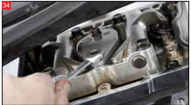
With a 3/8" wrench, loosen the two bolts holding the breather assembly.
