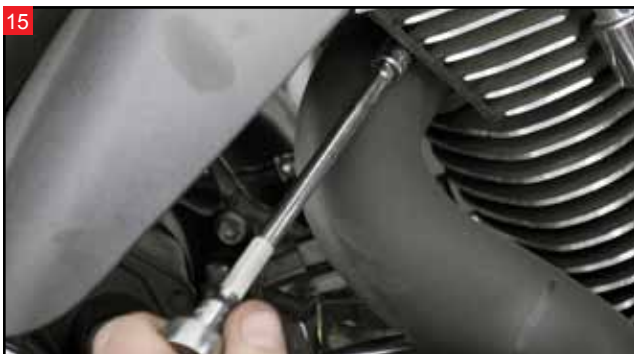
After removing the hardware holding the exhaust to the transmission bracket, remove the exhaust flange nuts with a 1/2" socket.
