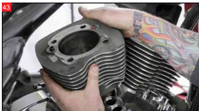
43 Raise the cylinder up and off the cylinder studs. It helps to keep the motorcycle in gear with the rear wheel on the lift to prevent the piston from moving while raising the cylinder.
