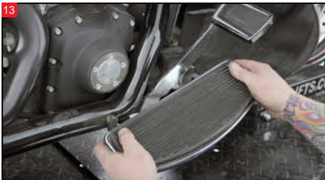
Remove the floorboard from the mounting brackets.
