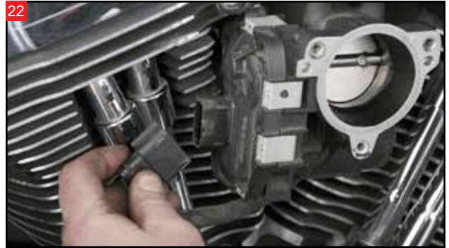
Disconnect the wiring from the servomotor on the throttle body.
