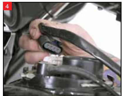
4 Disconnect the wiring for the fuel pump and fuel level sending unit.
