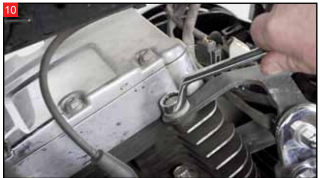
Remove the two bolts holding the horn mount/top motor bracket with a 9/16" wrench.
