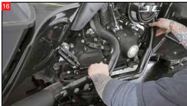
Remove the exhaust system from the motorcycle.
