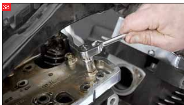
Loosen the six bolts holding the lower rocker housing to the head.
