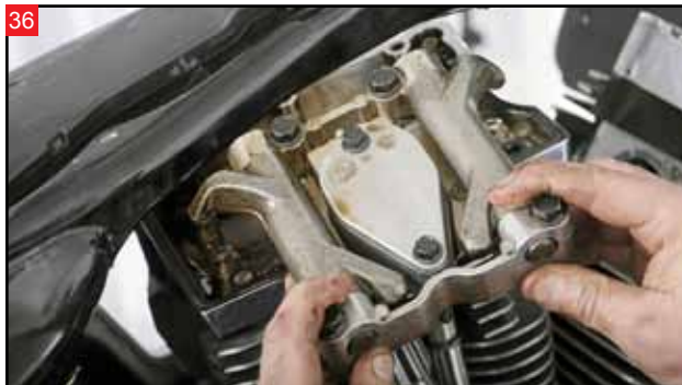
Remove the rocker arm pedestal from the lower rocker box housing.
