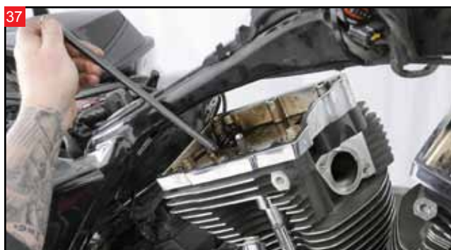
37 The pushrods and tubes are removed next. Repeat the process for the second cylinder, ensuring it is at TDC of the compression stroke when performing work.
