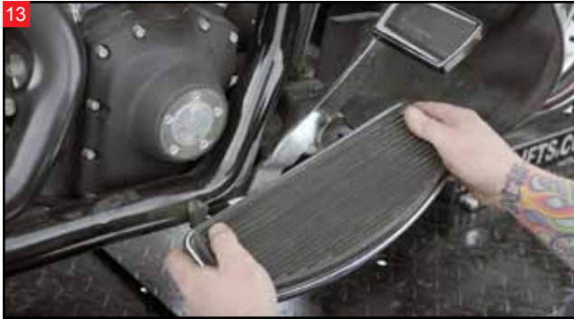
Remove the floorboard from the mounting brackets.
