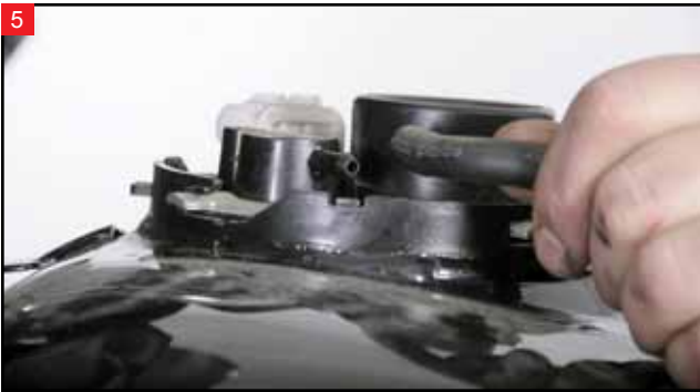
Unplug the vent line from the top of fuel tank.
