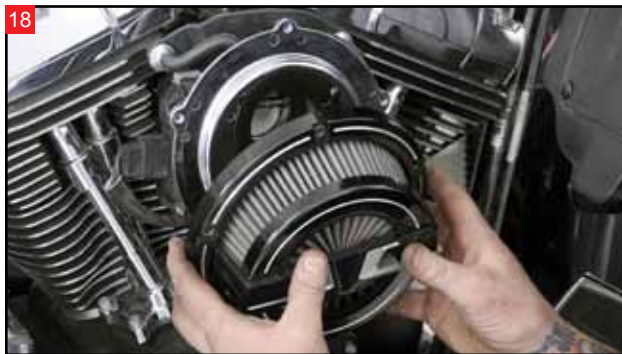
Remove the air cleaner filter and outer cover from the backing plate.
