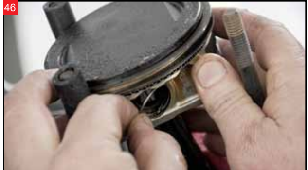
46 Use a small flathead screwdriver to remove the wrist pin retaining clip from the piston. Wear eye protection during this step.
