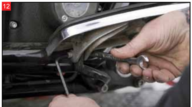
With a 3/16" Allen and 7/16" wrench, remove the floorboard mounting hardware.
