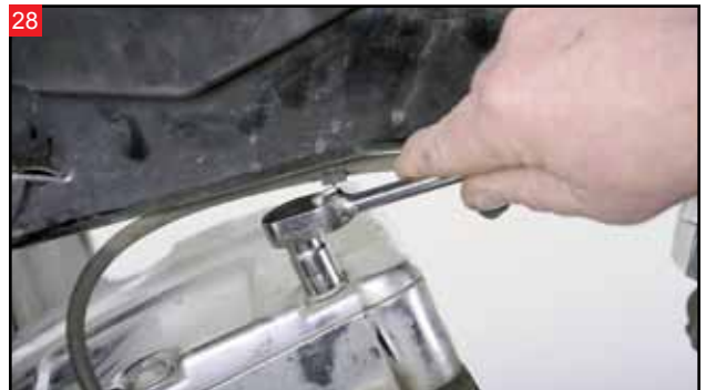
Using a 7/16" socket, remove the six bolts holding the rocker box top.
