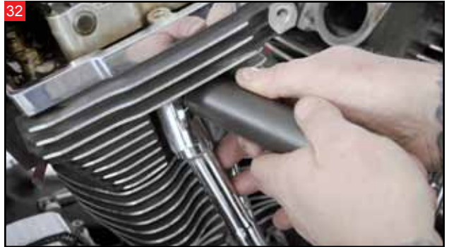
To access the pushrods, remove the top clips from the pushrod tubes. Use a center jack under the frame to raise the rear wheel off the lift.
