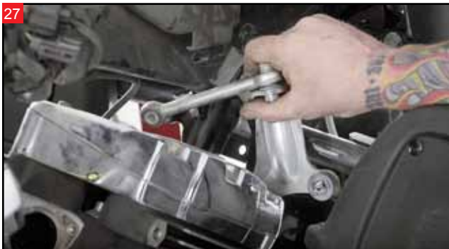
The front motor bracket can be taken off after removing the two bolts with a 9/16" wrench.
