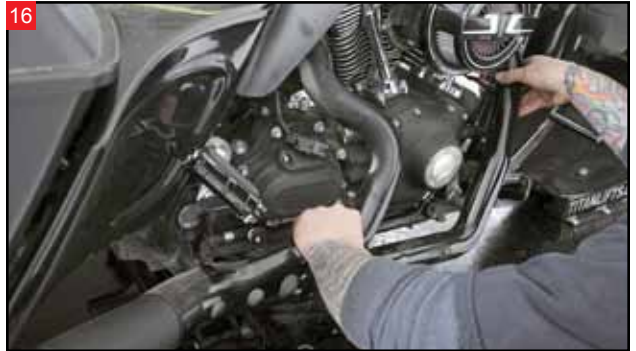
Remove the exhaust system from the motorcycle.
