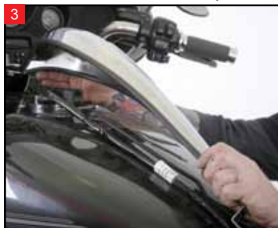
3 Remove the dash from the top of the fuel tank.
