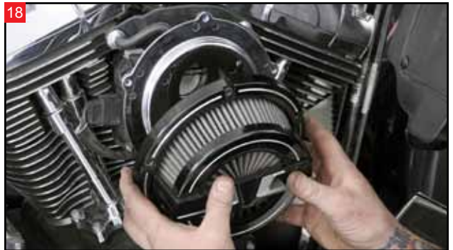
Remove the air cleaner filter and outer cover from the backing plate.
