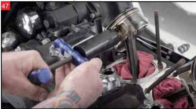
47 Use the wrist pin removal tool to clear the wrist pin from the connecting rod.
