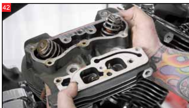
Lift the cylinder head up and off the cylinder. Repeat the process for the other cylinder head.
