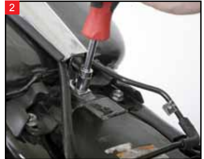
2 Remove the hardware holding the dash to the fuel tank.
