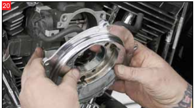
Remove the backing plate and breather hoses.
