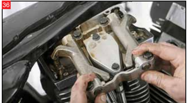
Remove the rocker arm pedestal from the lower rocker box housing.
