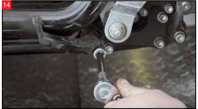
Use a 5/16" Allen to remove the bolt holding the right rear floorboard-mounting bracket.
