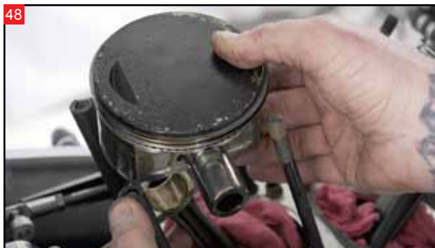
48 Remove the piston from the connecting rod. Maintain control of the connecting rod to prevent it from damaging the spigot of the engine case.
