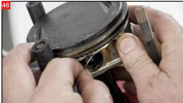
46 Use a small flathead screwdriver to remove the wrist pin retaining clip from the piston. Wear eye protection during this step.
