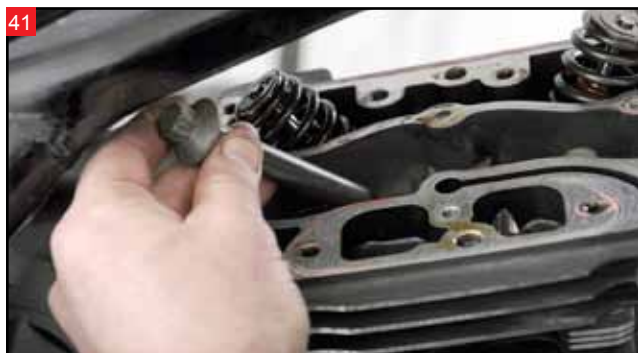
41 Remove the head bolts from the cylinder studs.
