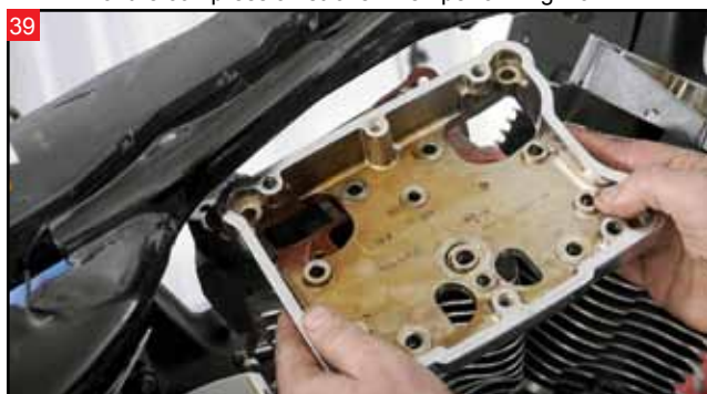
Remove the lower rocker housing from the cylinder head.
