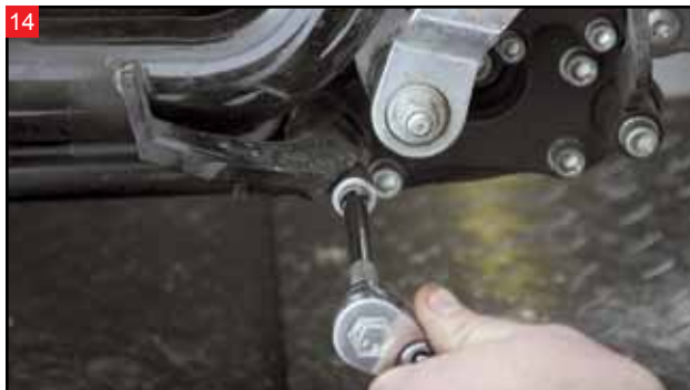
Use a 5/16" Allen to remove the bolt holding the right rear floorboard-mounting bracket.
