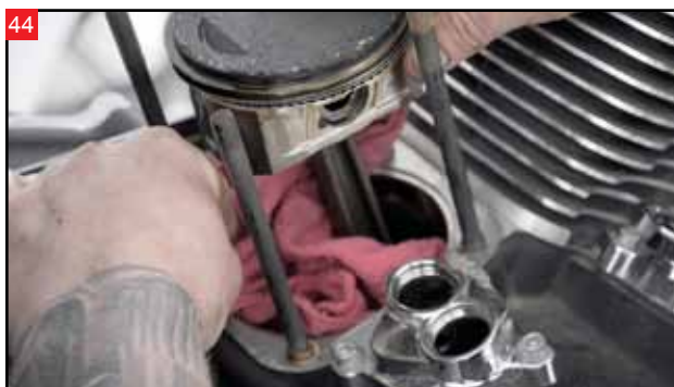
44 Place clean shop rags in the case spigot. This is to prevent the wrist pin from falling in the engine case when it is removed.
