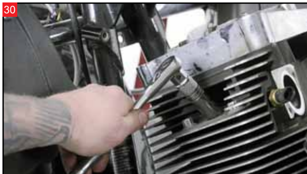
Remove the spark plugs from each cylinder head.
