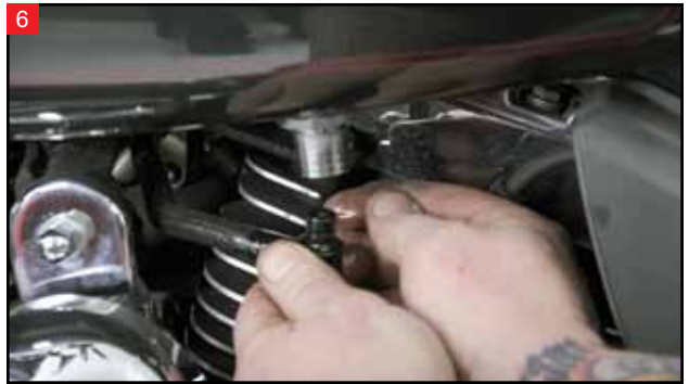
Disconnect the fuel line fitting from the quick-connect on the left lower side of the fuel tank.
