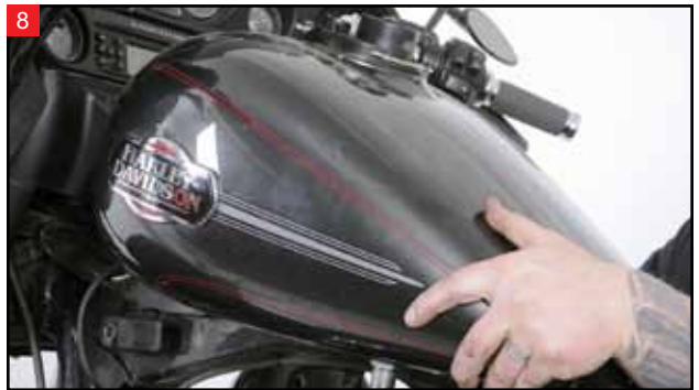
Lift the fuel tank up and off the backbone of the motorcycle.
