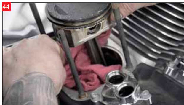
Place clean shop rags in the case spigot. This is to prevent the wrist pin from falling in the engine case when it is removed.
