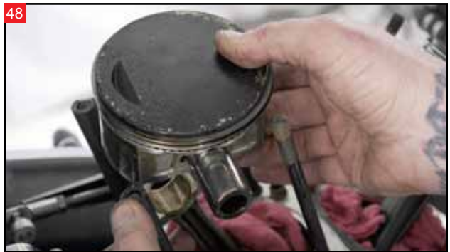
48 Remove the piston from the connecting rod. Maintain control of the connecting rod to prevent it from damaging the spigot of the engine case.
