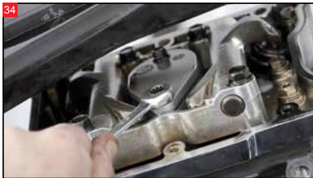
With a 3/8" wrench, loosen the two bolts holding the breather assembly.
