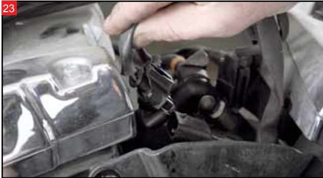
Unplug the connectors from the fuel injectors and sensors on the throttle body.
