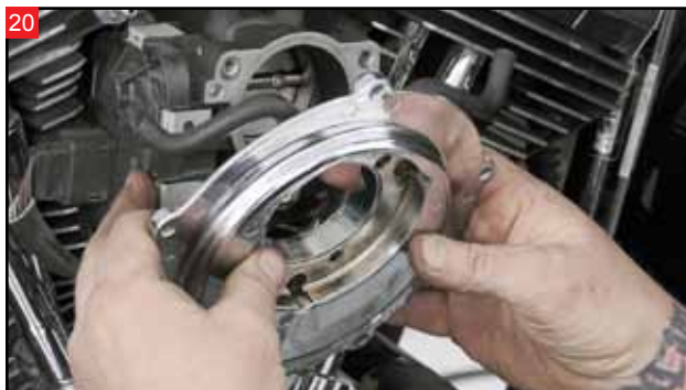
Remove the backing plate and breather hoses.
