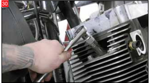
Remove the spark plugs from each cylinder head.
