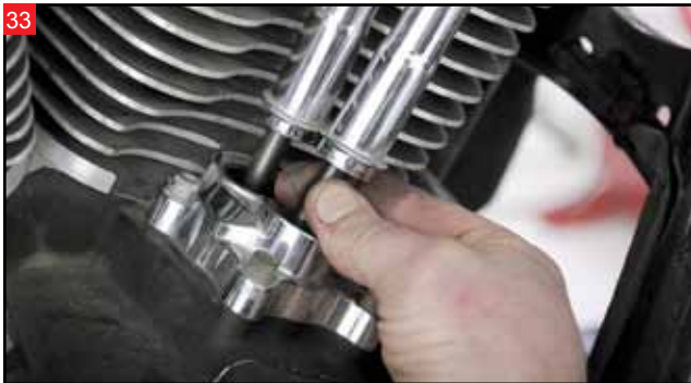
Put the transmission in sixth gear. Rotate the motor until the piston of the cylinder you are working is at TDC (top dead center) of the compression stroke. Verify the pushrods of that cylinder rotate freely by hand.
