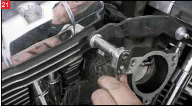
Use a 7/16" deep well socket to remove the breather bolts from the cylinder heads.
