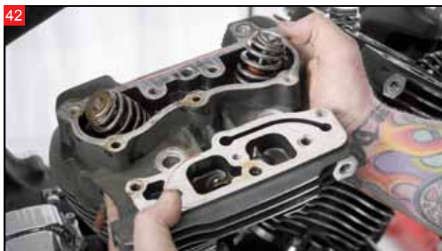
42 Lift the cylinder head up and off the cylinder. Repeat the process for the other cylinder head.
