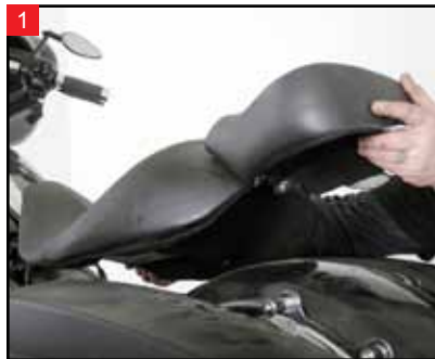
1 Remove the seat from the motorcycle. Disconnect the negative terminal from the battery.
