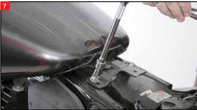
Use a T40 Torx to remove the four mounting bolts for the fuel tank.
