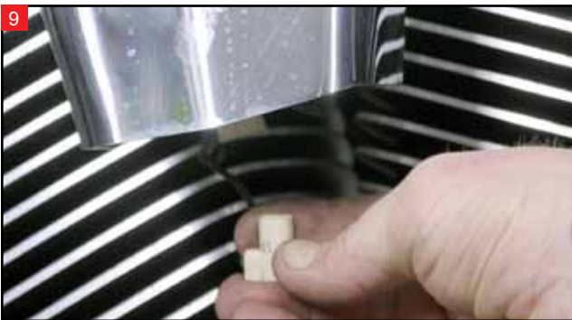
Unplug the positive and negative wires for the horn.
