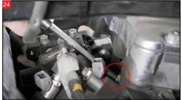
With a long 1/4" Allen, remove the two right side bolts holding the throttle body to the heads. The left side bolts are loosened using a 1/2" wrench.
