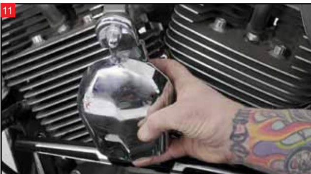
The top motor bracket can be removed from the cylinder heads.
