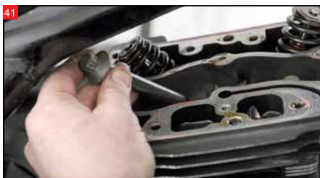
Remove the head bolts from the cylinder studs.
